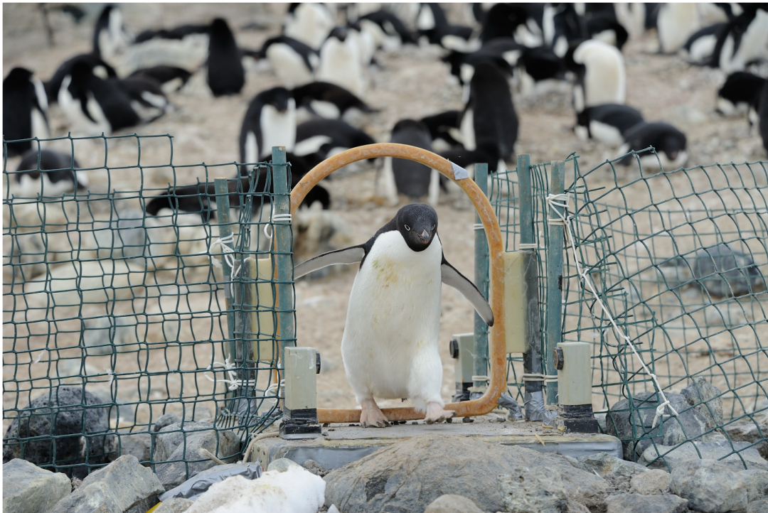
"Automated weighbridge for Adélie penguins" - journal.pone.0085291.g002" by Lescroël, A. L.; Ballard, G.; Grémillet, D.; Authier, M.; Ainley, D. G. (2014) - Lescroël, A. L.; Ballard, G.; Grémillet, D.; Authier, M.; Ainley, D. G. (2014). "Antarctic Climate Change: Extreme Events Disrupt Plastic Phenotypic Response in Adélie Penguins". PLoS ONE 9: e85291. DOI:10.1371/journal.pone.0085291. Licensed under CC BY 4.0 via Wikimedia Commons
